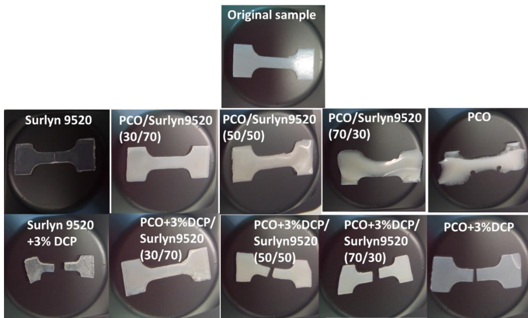
Figure 4.60. Dog-bone shaped samples after self-healing experiment for all developed samples (plus the original sample).
