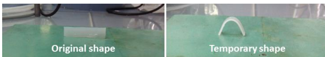
Figure 3.20. Original and temporary shapes of a gamma irradiated PCO sample.
