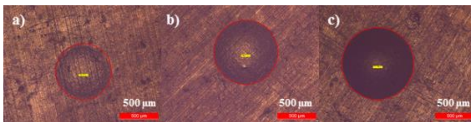
Figure 4.39. Diameters measured by optical microscopy of the holes in Surlyn 1705 + PCO + 3% DCP sample with a) 5 N, b) 10 N, c) 15 N.
