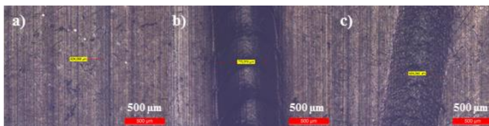
Figure 4.42. Widths measured by optical microscopy of the lines in Surlyn 8940 + PCO + 3% DCP sample with a) 5 N, b) 10 N, c) 15 N.
