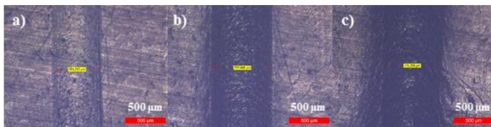
Figure 4.41. Widths measured by optical microscopy of the lines in Surlyn 1705 + PCO + 3% DCP sample with a) 5 N, b) 10 N, c) 15 N.
