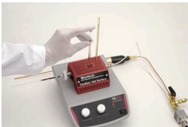
Figure 3.6. The Adsorbent Tube Injector System (ATIS) (source: Sigma-Aldrich, 2016).
