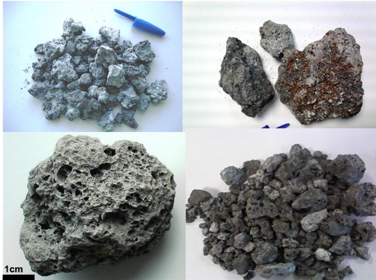
Fig.3.3. Images of some treated and non treated black steel slag. (a) M1T, (b) M2, (c) M4 and (d) M2T.
