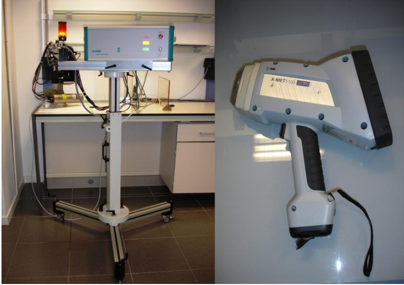
Fig.3.6. X-Ray Fluorescence (XRF) instruments. ArtTax portable Micro-Energy Dispersive X-Ray Fluorescence ( \mu -EDXRF) equipment on the left and the handheld Electron Dispersive X-Ray Fluorescence (EDXRF) analyzer on the right.
