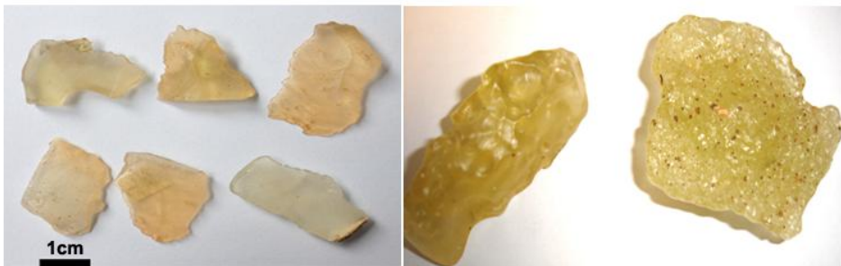
Fig.3.1. Studied Libyan Desert Glasses belonging to the Meteorites Collection of the Basque Country University (UPV/EHU).
