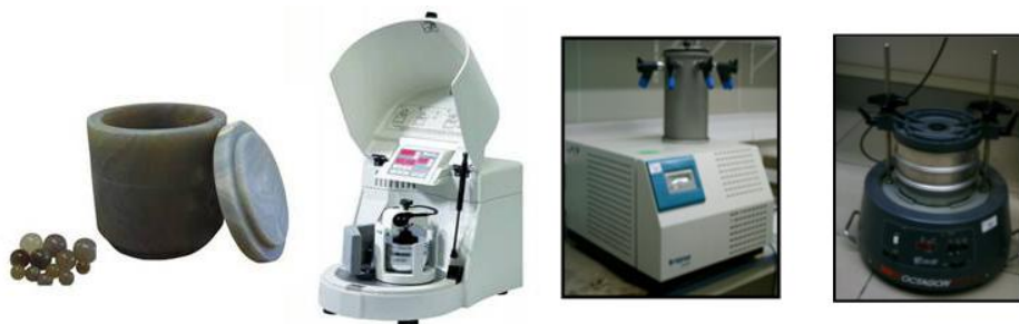
Fig.3.5. Images of the agate ball mill, the mill, the lyophilizer and the sieve shaker.
