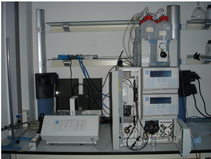
Fig.3.12. Dionex ICS 2500 Ion Chromatographic system with an ED50 conductivity detector coupled to an AS40 autosampler.
