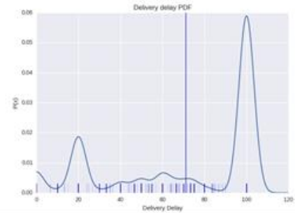
Figure 3: Simulation output graphic example (Delivery delay PDF), with LRU algorithm and LCE placing algorithm.
