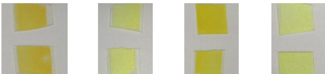
Figure 3.16. Photographs of the mesoporous films of TiO 2 sensitized with the dyes A15 , B15 , A16 and B16 .
