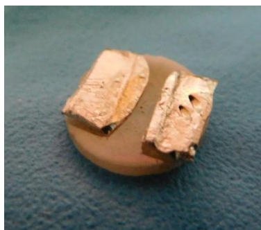
Figure 6.3: Lateral configuration for lithium plating/stripping experiments using the currently-developed garnet ceramic (Ga 0.15 :LLZO) and two parallel strips of lithium foil to serve as electrodes and lithium sinks.
