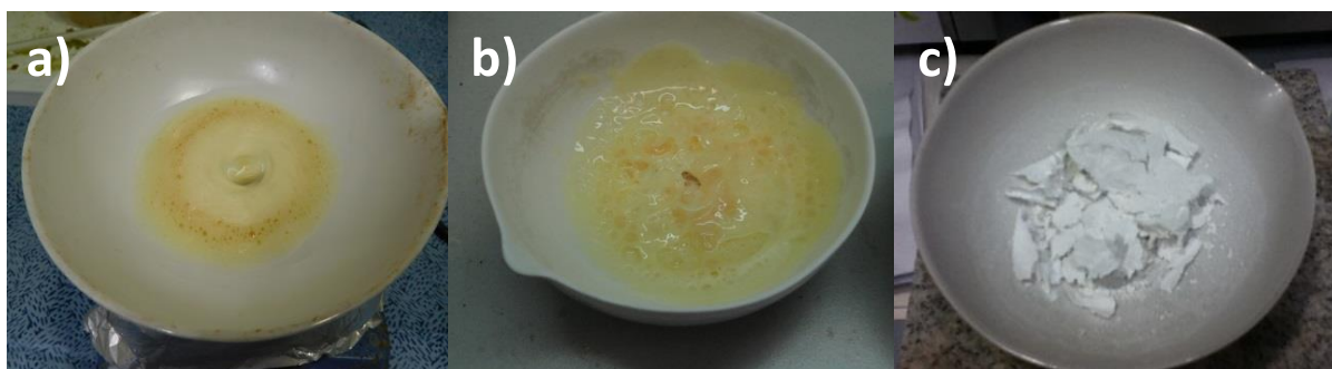
Figure 2.1: A sol-gel route preparation (citrate-nitrate type): a) reagent nitrates are dissolved in a citric acid solution, b) the water component is minimized via heat-driven evaporation until a gel forms, and c) furnace combustion at a relatively low temperature (e.g. 600°C) to burn off a large portion of organics, In preparation for crystalline phase-formation in a subsequent calcination step.
