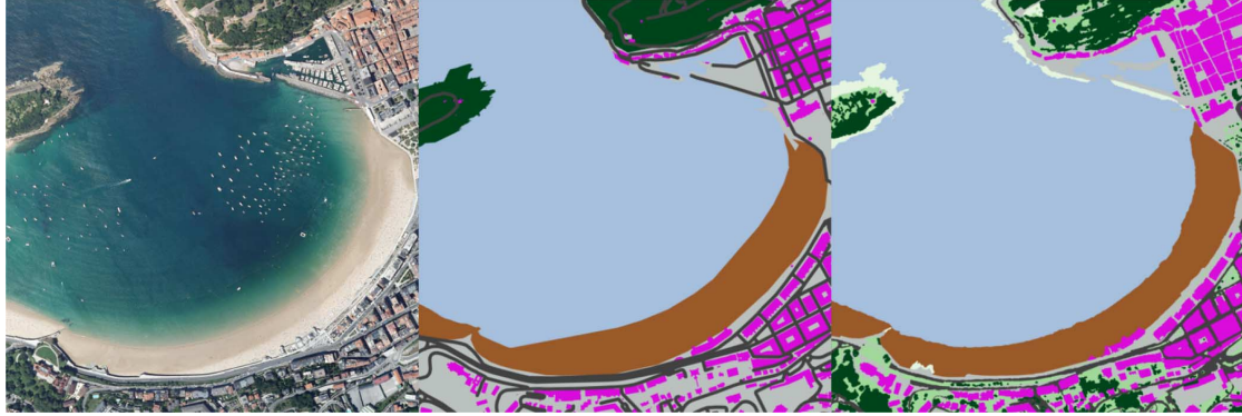
Fig. 8. From left to right: original image, pre-existing vector-map-based ground truth, manually produced pixel-level image interpretation-based ground truth for the La Concha test site. The subset of the defined ground cover classes includes eight elements from the original 12: building (purple), sea (blue), bare soil (light green), pasture (green), woodland (dark green), street (gray), urban roads (dark gray), and beach (brown). An increased level of detail is evident, particularly, in vegetated areas between buildings and near to Bare Soil areas.
