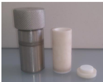
Figure 3.1. Teflon liner and stainless steel autoclave used for the synthesis of aluminophosphate materials.
