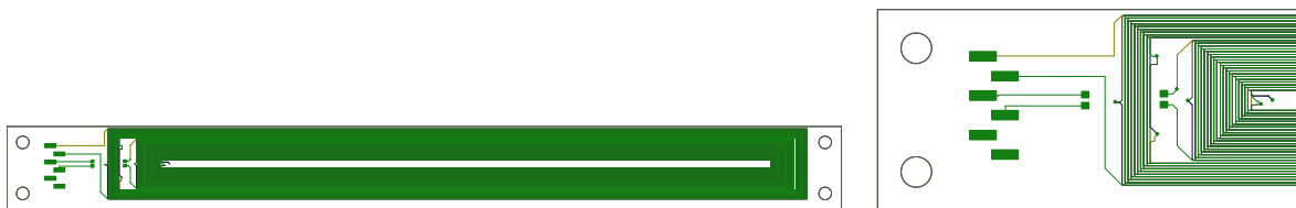
Figure 11.4 – Example of a coil designed by the author for the measuring of small aperture PMQs. Left, global view. Right, detail of the connection side, showing the vias structure of the PCB.
