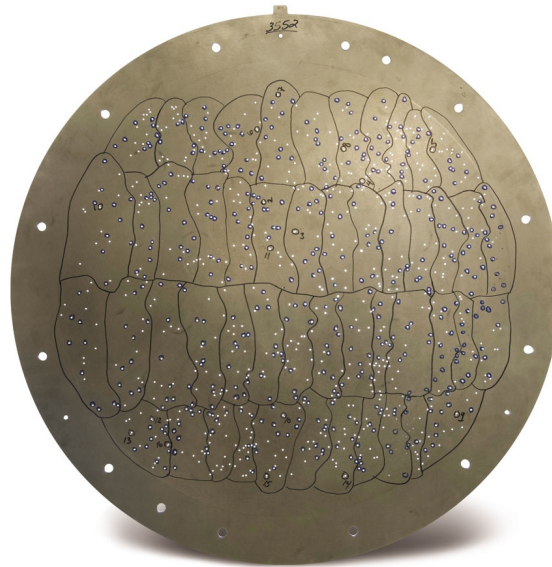
Figure 3.2: Left: the optical camera of the SDSS-III survey, composed of an array of 30 CCDs with 2048 \times 2048 pixels each. The filters correspond to the five colour-bands u , g , r , i and z . Right: One of the plates used in the BOSS survey. The holes in the plate indicate the positions in the sky of the objects whose redshift is measured placing optic fibers that conduct the light to the spectrograph. The equivalent diameter sizes in the sky of the plate and the fibers are 3 degrees and 2 arcsec, respectively.
