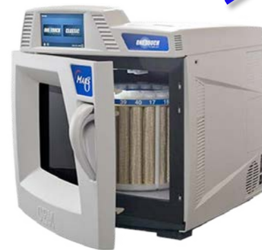
Microondas CEM MARS-5 160 °C; 2 h
