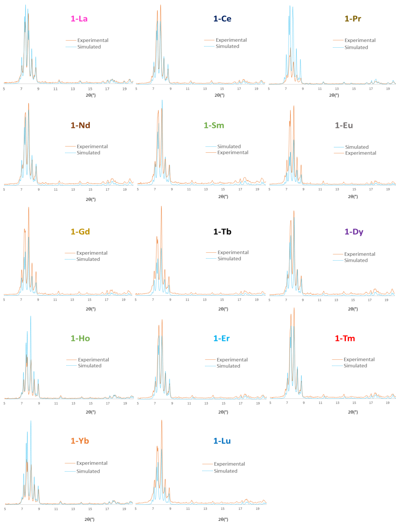
Figure A3.6. Comparison between the experimental powder X-ray diffraction patterns of 1-Ln compounds with the corresponding simulated PXD patterns from single-crystal X-ray diffraction data.
