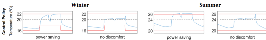
Figure 4.11. Influence of the weights in the cost function. Winter and summer responses for an energy saving and tracking setpoint policies. Figure also shows the comfort band temperatures for each season.
