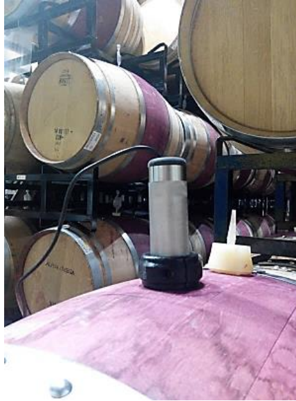
Figure 5.3-3: Wine-NIR prototype immersed in a barrel through the cork hole.
