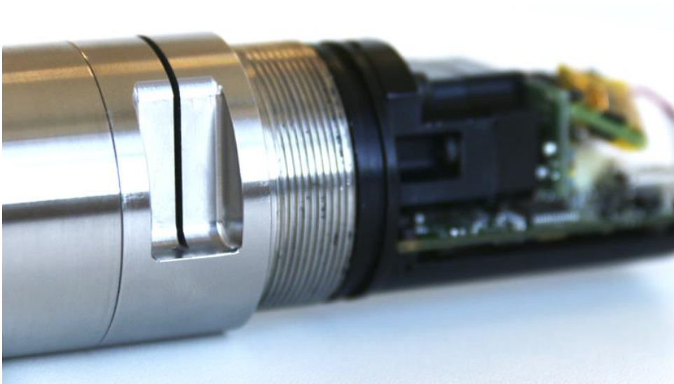
Figure 5.3-2: Detail of the NIR prototype, with the 1 mm slit designed to be filled by capillary forces of the fluid.
