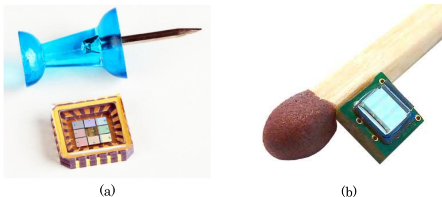
Figure 1.4-4. Filter array and 2D photo-detector array based VIS-NIR micro-spectrometers. (a) PixelTEQ's PixelSensor™. (b) Espross's SPM64-NIR.
