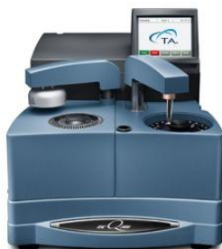
Figure 2.4 DSC Q2000 from TA Instruments used to measure the calorimetric response.
