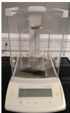
Figure 2.17 Analytical balance and density kit used for the density calculation.
