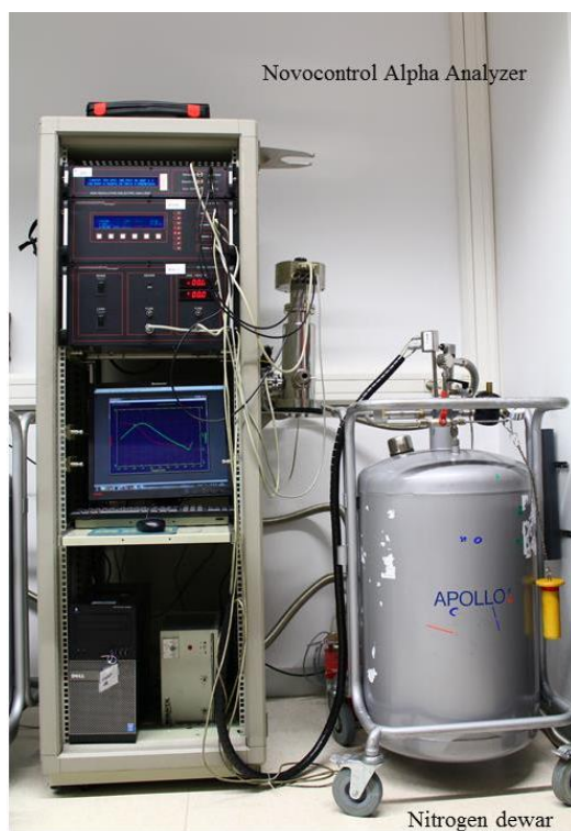
Figure 2.10 Novocontrol alpha analyzer and nitrogen Dewar.
