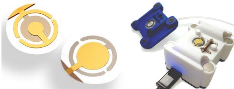
Figure 1.2. Both sides of a quartz crystal resonator and a quartz crystal microbalance system.
