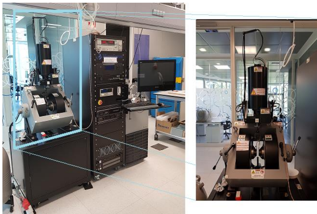
Figure 2.8. Vibrating Sample Magnetometer located at BCMaterials used to obtain the hysteresis loops.
