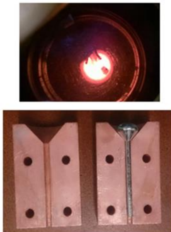
Figure 2.3. The melted alloy and the obtained ingot inside the copper mould.
