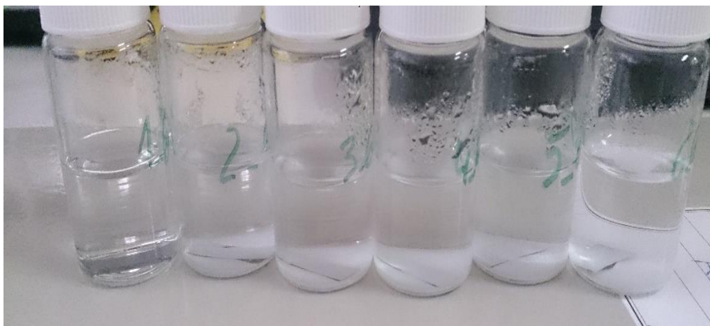
Figure 4.10. Precipitate formation and deposition that takes place after de reaction process for increasing concentration of zinc reactant in samples 1_63 to 6_63.
