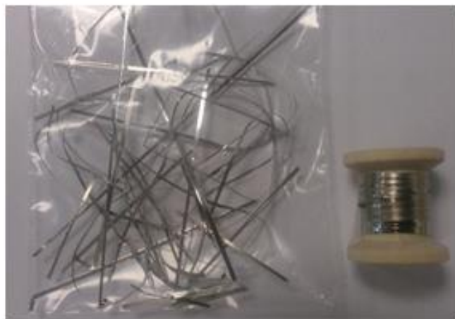
Figure 2.5. View of the Fe_{54}Ni_{24}Cr_2Si_{10}B_{10} amorphous ribbon obtained by the melt spinning technique.
