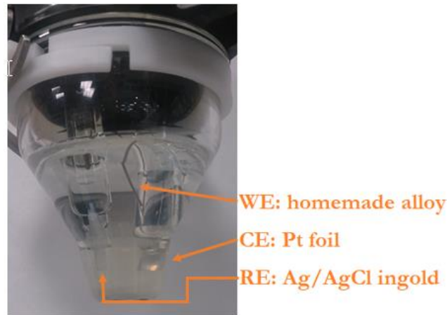
Figure 2.20. Cell used for the corrosion experiments with the three electrodes on it.
