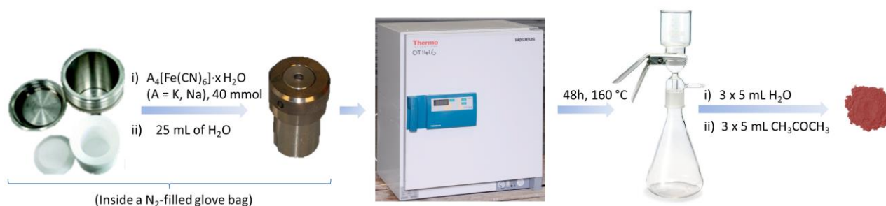
Figure 3.36. Schematic synthesis procedure for preparing A-PW (A = Na, K), A_{2-x}Fe^{2+}_{1+(x/2)}[Fe^{II}(CN)_6] \cdot yH_2O , by hydrothermal method, following Jiang's methodology.
