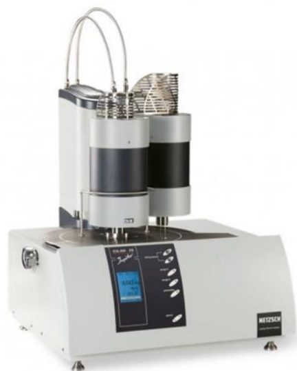
Figure 2.4. Thermogravimetric analyzer TGA NETZSCH STA 449 F3 Jupiter.
