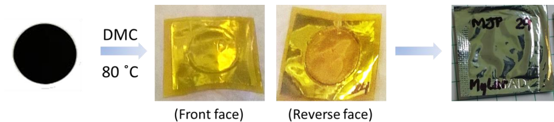
Figure 2.11. Detailed scheme for electrode (13 mm of diameter) preparation for the ex-situ XAS measurements.
