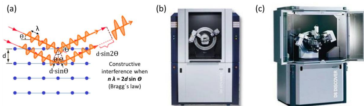
Figure 2.1. a) Schematic description of the diffraction of lattice planes, following Bragg's law, b) Bruker D8 Advance diffractometer and c) Bruker D8 Discover diffractometer deployed in this work.
