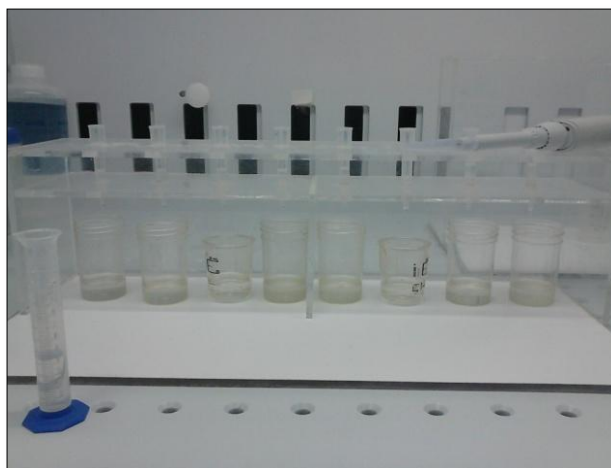
Figure 4. The solutions were loaded into cation exchange columns filled with Sr.spec ® (EiChroM industries, Dariel, IL, USA), a strontium selective resin.
