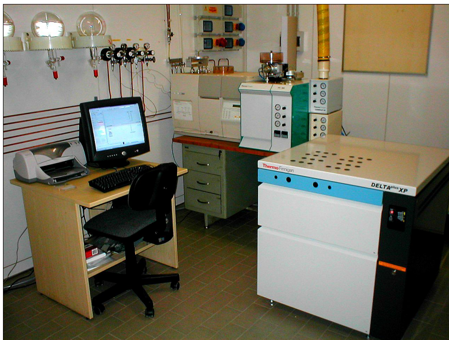
Figure 7. Thermo Finnigan TCEA coupled to a Delta Plus XP Spectrometer at the University of Parma (give up by Paola Iacumin and Enrico Maria Selmo, Università degli Studi di Parma).
