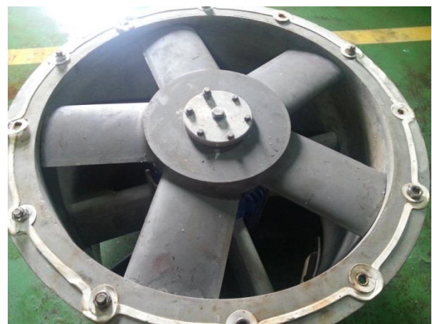
Figure 3. Wells turbine in NEREIDA MOWC wave power plant.
