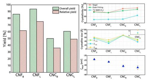
Fig. 6. Left: Yields of the elaborated nanoparticles, overall yield corresponds to the amount of CNC/CNF obtained for each 100 g of cellulose, relative yield corresponds to the amount of CNC/CNF obtained related to the cellulose content as calculated by TAPPI methods Right: Crystallinity indices, crystallite domain sizes and zeta potential of the elaborated nanoparticles.
