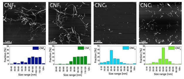
Fig. 5. AFM images of the elaborated cellulose nanoparticles. The lower part of the figure presents the corresponding size ranges as obtained with the Nanosizer.
