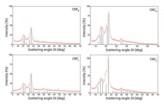
Fig. 7. Powder diffraction patterns (red scatter) as well as main diffraction signals as obtained from 2nd Derivate fitting (black lines) all values are normalized to the intensity of the 200 plane of the CNC<sub>L</sub>. (For interpretation of the references to colour in this figure legend, the reader is referred to the web version of this article.)
