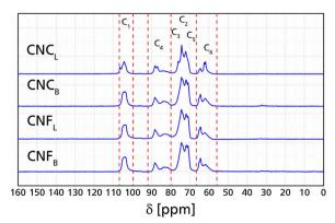
Fig. 8. NMR analysis of cellulose nanoparticles.
