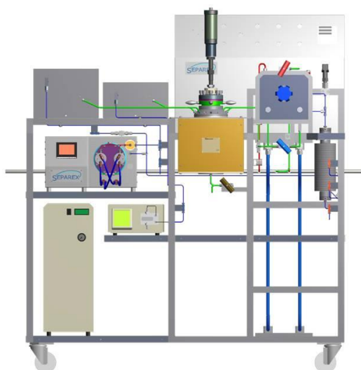
Figure II.1-4: Supercritical batch reactor scheme.
