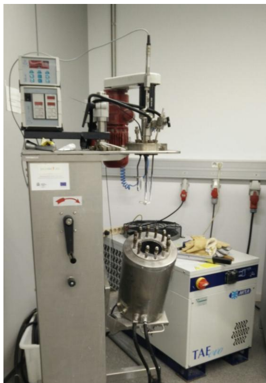
Figure II.1-1: Subcritical hydrothermal batch reactor.
