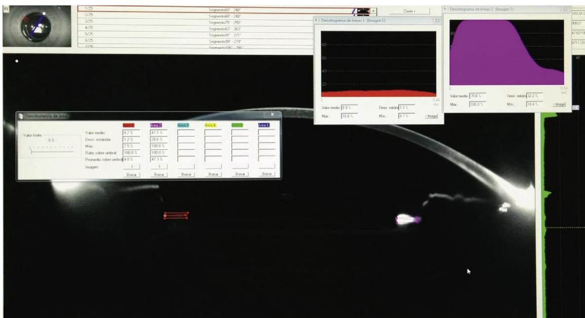
Figure 1. Assessment of area, linear, and peak densitometry measurement at a selected meridian using the Scheimpflug device software. The peak densitometry value appears automatically on the right side of the screen.
