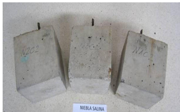
Figure 14: Corrosion rate in both types of concrete after a saline fog test. Image of samples after the test
