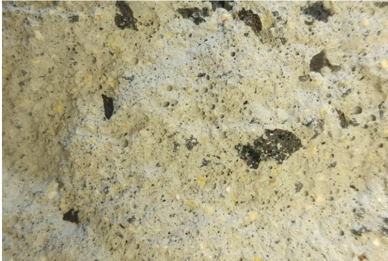
Figure 7: Mix SC3 showing high spherical porosity.
