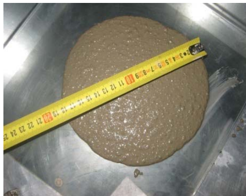
Figure 3.4: Measuring of mortar spread
