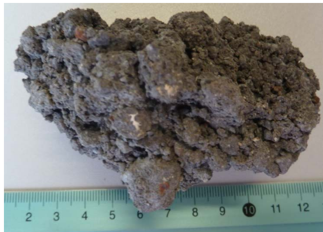
Figure 3.2: Electric arc Furnace slag particle
