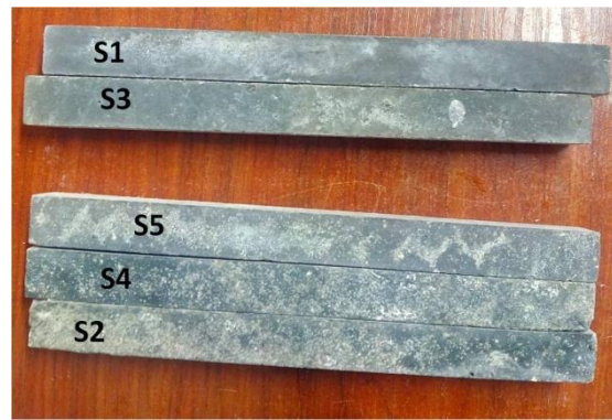
Figure 9: Samples after immersion in water at 70°C.
