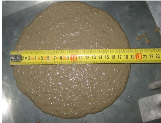
Figure 3: Spreading of the mixture S4 in the mini slump cone
