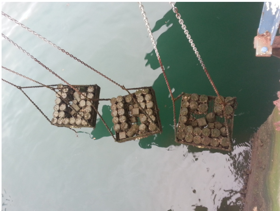
Figure 3.8: Specimens cages at tidal zone
