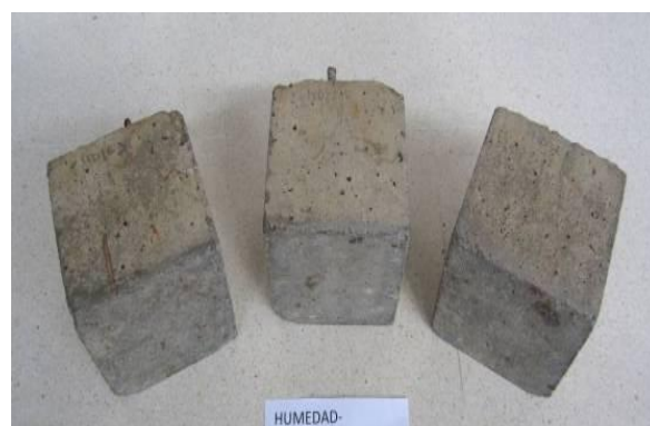
Figure 13: Corrosion rate in the two types of concrete after wetting-drying test. Image of EAF slag samples after the test
