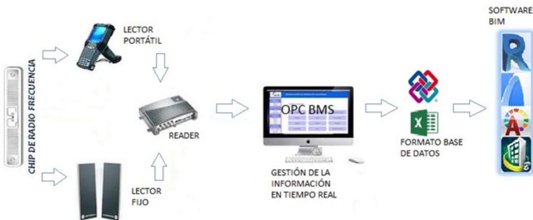
Fig. 6. Flujo RFID – OPC BMS – BIM ( http://www.sigigan.com/rfid.html ) RFID – OPC BMS – BIM flow ( http://www.sigigan.com/rfid.html )
