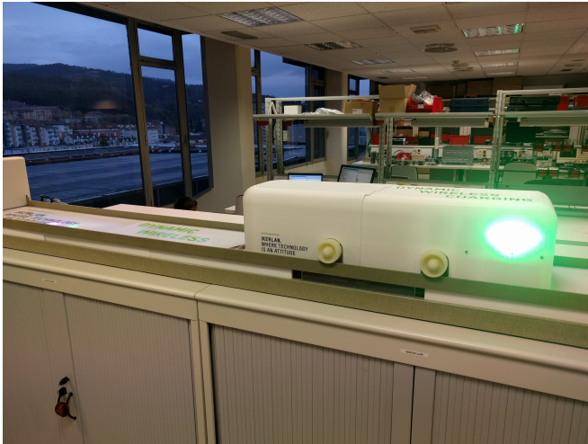
Figure 3.18: 50W small-scale three-phase IPT charger.
