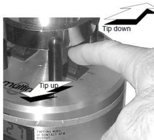
Figure 24: tip and sample approach buttons [15]
