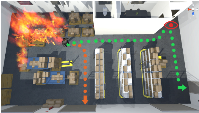
Figure 9: Fire in ground floor: evacuation options.
