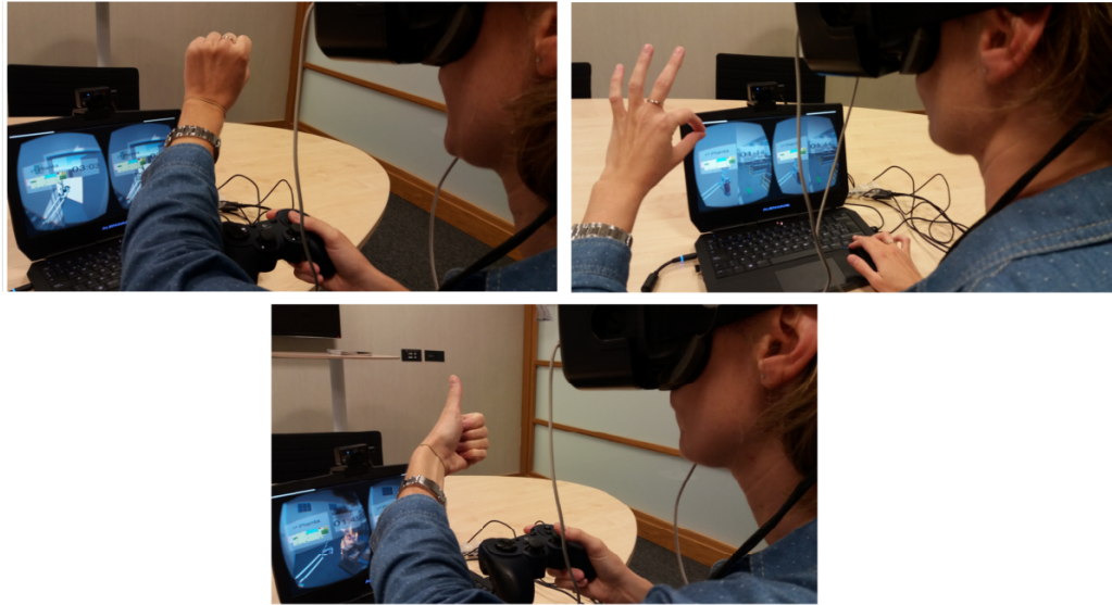
Figure 3.7: Leap Motion Controller used to detect hand gestures in PREST R&D project.
