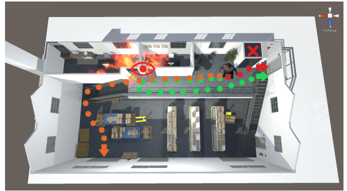
Figure 10: Fire in first floor: evacuation options.
