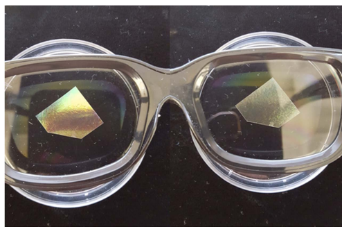
Figure 7. Observation of two CNC films through the two different lenses of 3D glasses (left-handed and right-handed circular polarisers).
