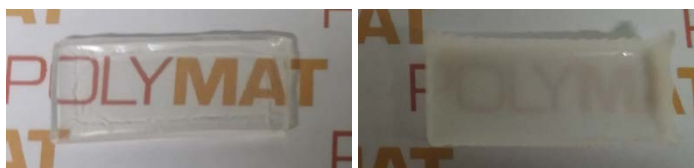
Figure 4.9. Polymer film of non-grafted PCD based (left) and PPG based (right) immersed one day in water
