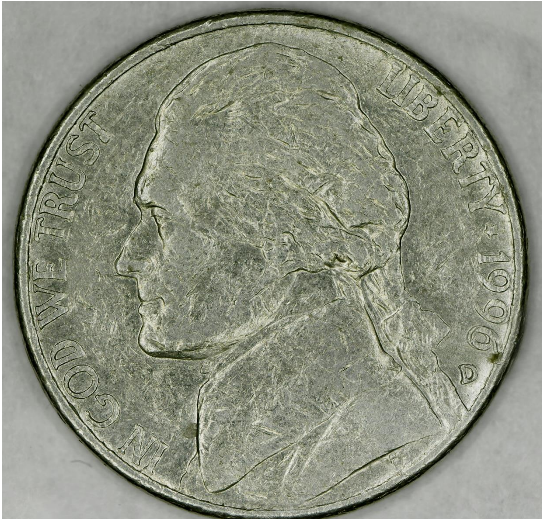
Figure 3.7. Image stitching results for a 16x18 images scan of a coin
