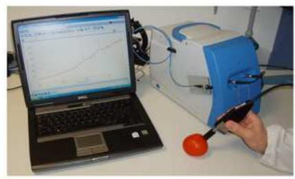
The portable and confocal Raman instruments using 514 and 785 nm laser excitation wavelengths provide different and complementary spectroscopic information about tomato fruits composition.
