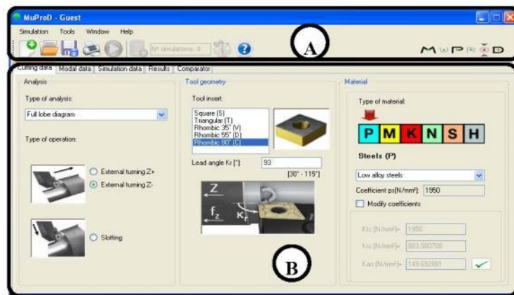
Figure 1. Example of the main machining interface window.
