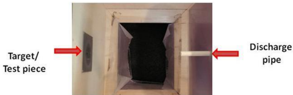
Figure 116. Gravelometer test layout
