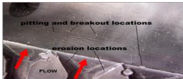
Fig 8. Breakout, erosion, and washout appears in the opposite locations of where they would be expected - on the low pressure side of the flowing liquid. [11]
