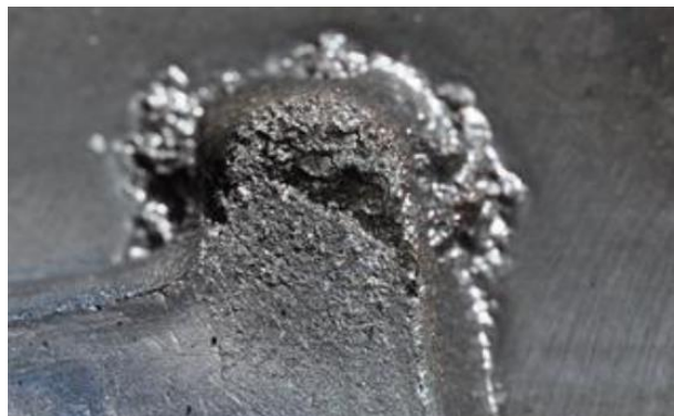
Fig 9. Typical Cavitation phenomena in High Pressure Die Casting of Aluminium Dies [6]
