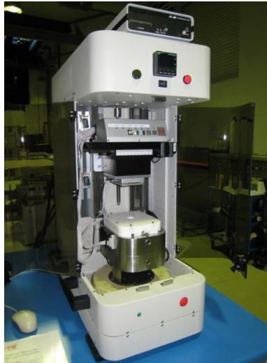
Figure 101. Universal Material Tester (UMT3 of CETR)
