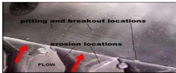
Figure 11. Breakout, erosion, and washout appears in the opposite locations of where they would be expected - on the low pressure side of the flowing liquid. [20]
