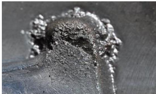
Figure 12. Typical Cavitation phenomena in High Pressure Die Casting of Aluminium Dies [12]
