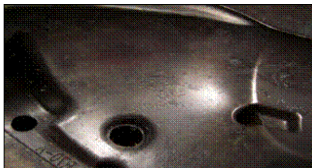
Fig 10. Exhibited sheet or cloud and vortex cavitation effect [11]
