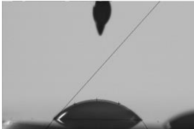
Figure 91. The contact angle calculation through 5 points measurements.
