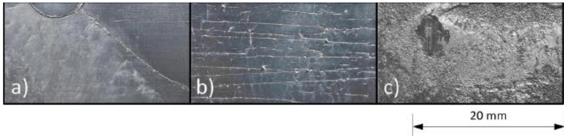
Figure 1. Detailed picture from tension cracks (a), heat checks (b) and washouts (c). [5]
