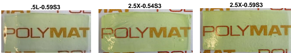
Figure 4. Films from the dispersions which show the broadest particle size distributions in Figure S9.
