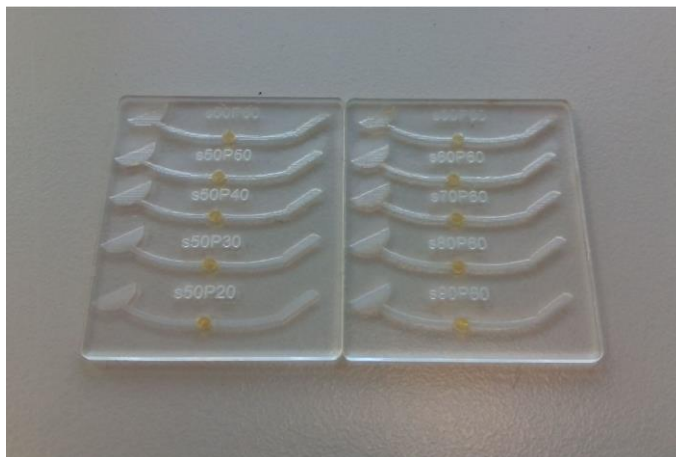
Figure 5.4: Evaluation of different depths and speeds (%) using the CO 2 ablation laser system. The ionogels were polymerised in the reservoirs.
