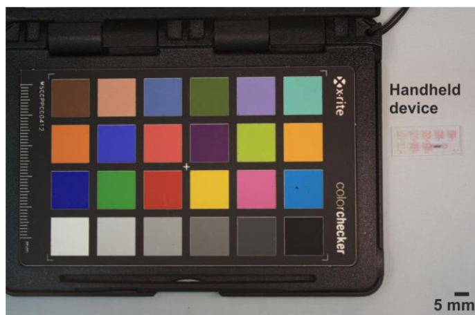
Figure 9.3: Picture of the device obtained using the X-Rite ColorChecker Passport card as the colour standard for further calibration.
