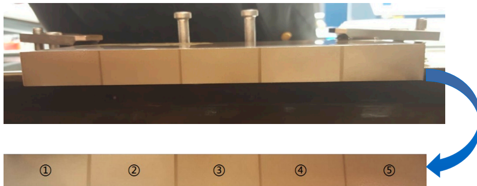
Figure 2. Regions on the workpiece during the experiments as a function of wire infeed.
