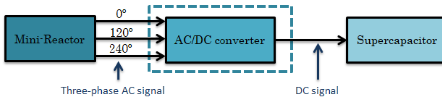
Figure 9-23: AC complete system with the harvester (mini-reactor), power management (AC/DC converter) and the storage device (supercapacitor).
