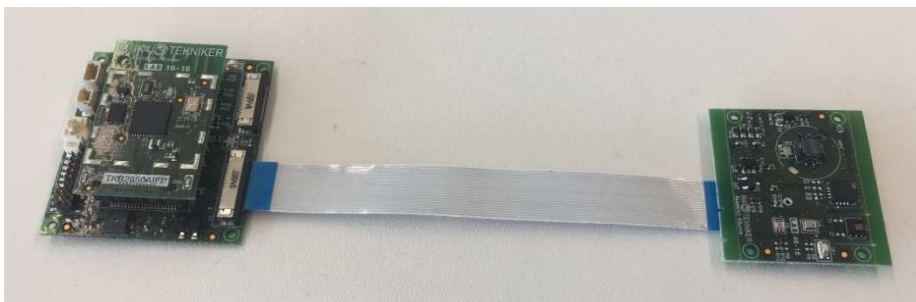
Figure 15-2: Wireless sensor network device which will be powered by future energy harvester system developed in this work.
