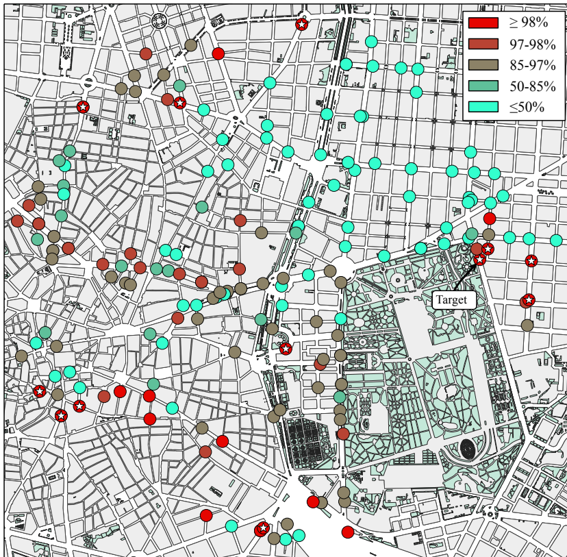
FIGURE 3.1: Automatic traffic recorders (ATRs) in the center of Madrid, colored by their data availability during 2014 (in % of valid 15-minute intervals over the year).
