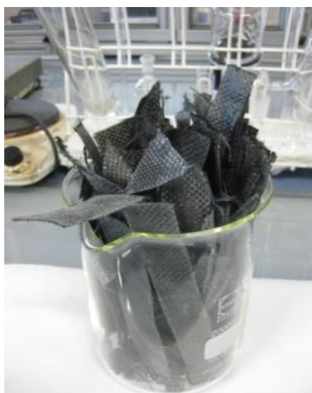
Figure 4. Residual CFRP sample before pyrolysis.
