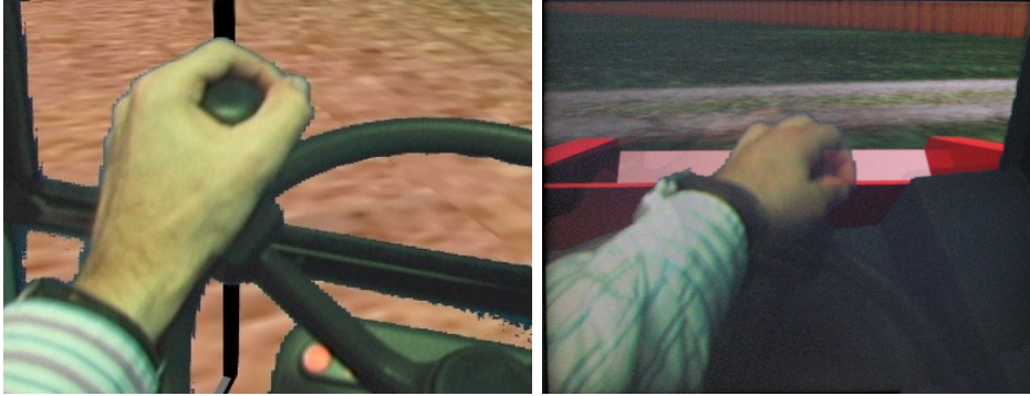
Figure 4.5: Chroma-key result as presented to the user in the HMD displays. Left: driving an excavator, Right: driving a dumper
