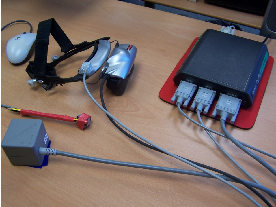
Figure 4.12: Hardware for the experimental manual welding simulator. The Z800 HMD with a magnetic sensor attached, a hand-held stick with a magnetic sensor (simulating the welding electrode holder) and the magnetic field emitter and control box.
