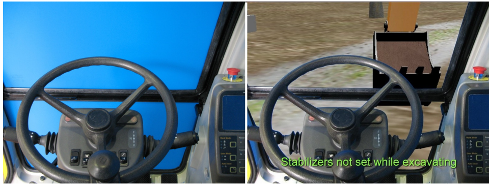
Figure 4.1: Simulated illustration of the chroma-key concept. Left: a view of the excavator cab with blue covered windows. Right: the view after chroma-key substitution of blue areas with virtual environment
