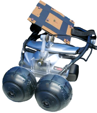
Figure 4.4: Experimental see-through HMD developed in the project. Two cameras are mounted in front and an active marker for pose tracking is seen at the top.
