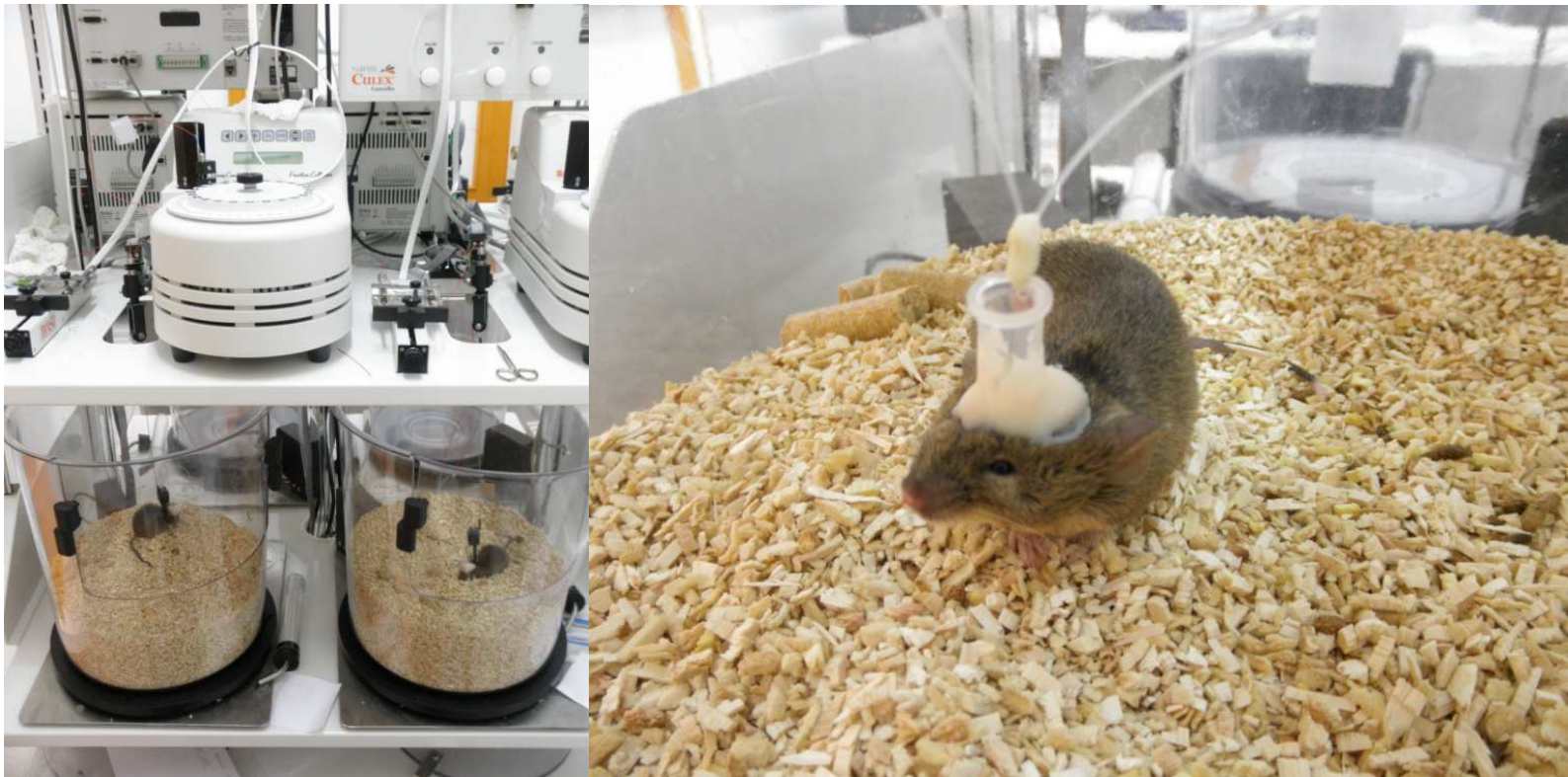
Fig. 26- Left photograph: BASi equipment used for microdialysis experiments in mice. Right photograph: 129/Sv strain mouse during microdialysis experiment.
