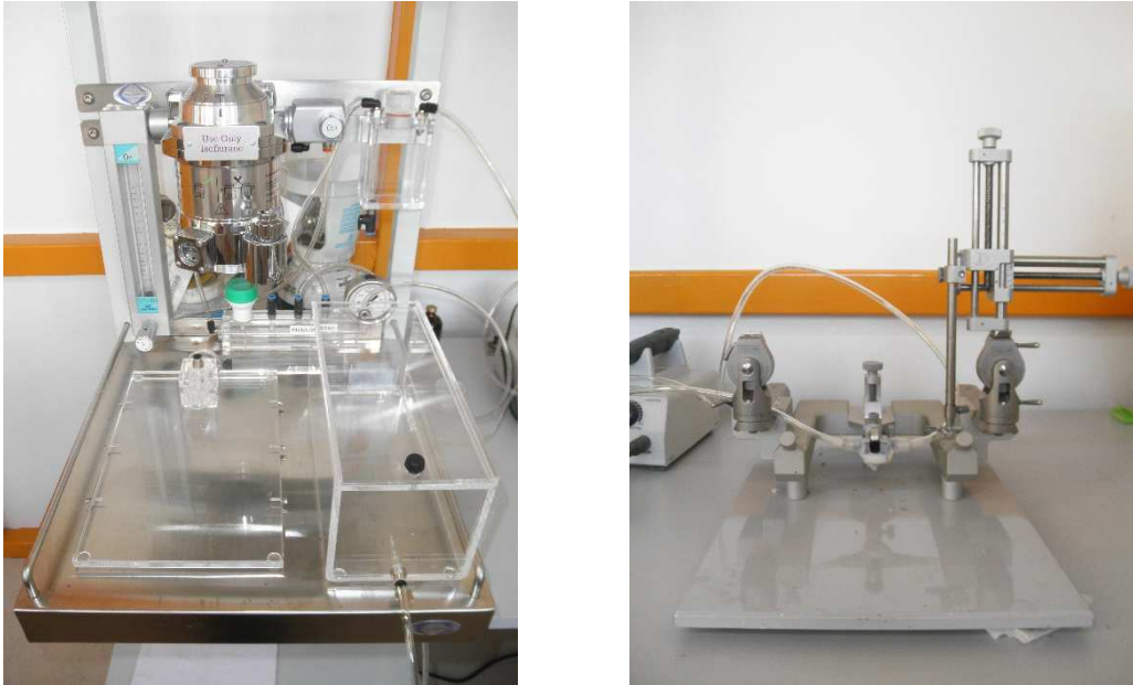
Fig. 19- Left panel: inhalation anesthesia system. Right panel: mouse mask for anesthesia maintenance coupled to the inhalation anesthesia system shown on the left.
