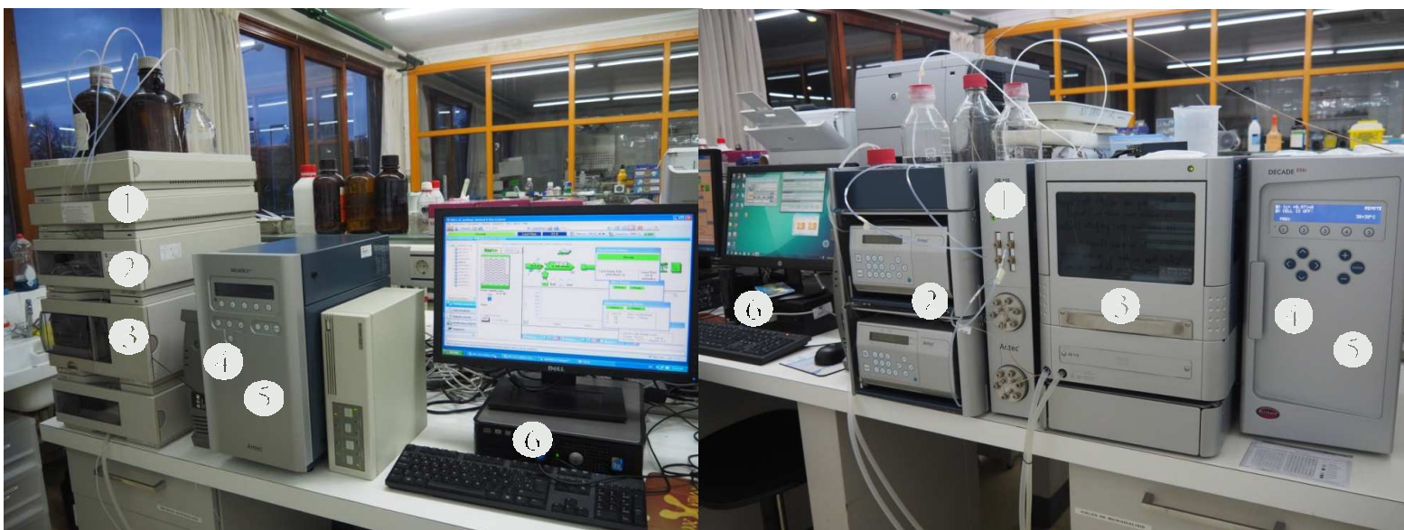
Fig. 34- Left panel: High-Performance Liquid Chromatography (HPLC) equipment coupled to an electrochemical detector. Right panel: Ultra-High Performance Liquid Chromatography (UHPLC) equipment coupled to two electrochemical detectors. 1=degasser; 2=pump; 3=autosampler; 4=chromatographic column; 5=electrochemical detector; 6=control station.
