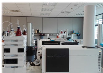
Fig. 4.20. LC-QTOF equipment used in this study.
