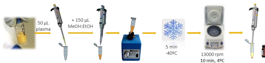
Fig. 5.8. Sample treatment for plasma protein precipitation and metabolite extraction.
