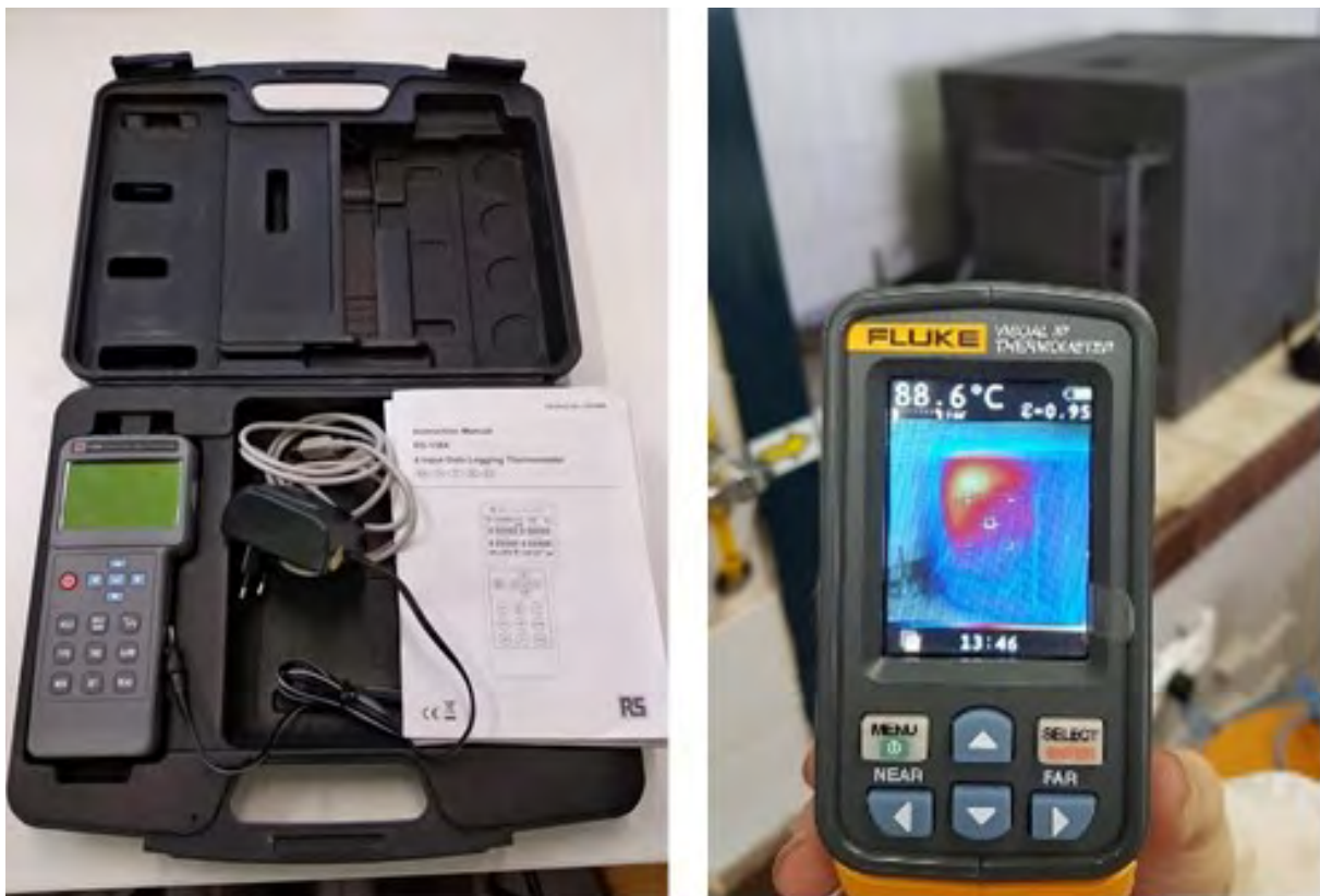
Figure 5. To calibrate the furnace, a temperature probe is used (left). An infrared thermal camera shows the thermal losses due to poor insulation (right)
