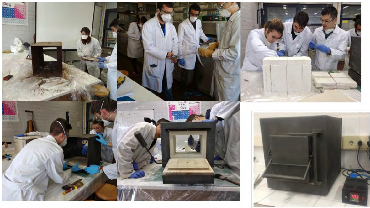
Figure 4. Different stages of the reconstruction process and final furnace ready for being calibrated
