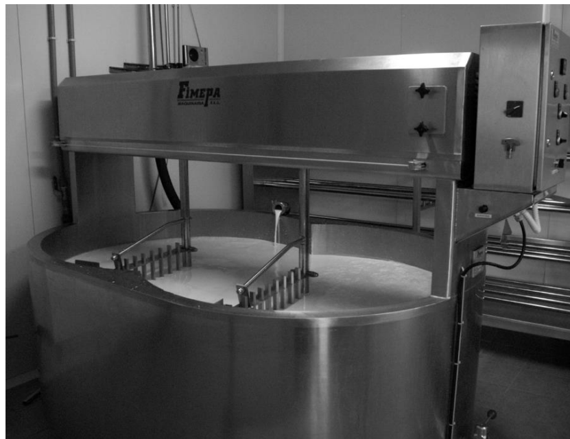
Figure IV.1. Double O-shaped vat with two fixed axes (Original photo: A. Aldalur).
