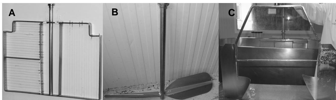
Figure IV.4. Cutting frame with vertically and horizontally arranged wires (A), helix-shaped (B) and irregular-shaped, (C) stirring tools used in small rural dairies (Original photos: A. Aldalur).
