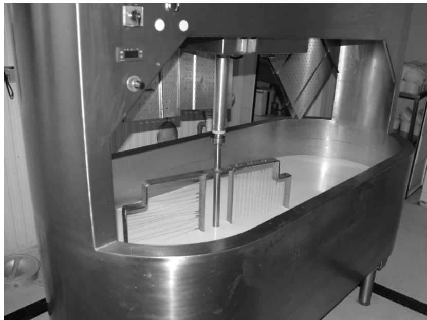
Figure IV.3. Oval-shaped vat with one axis of rotation and cutting frames with separately arranged vertical and horizontal wires (Original photo: A. Aldalur).
