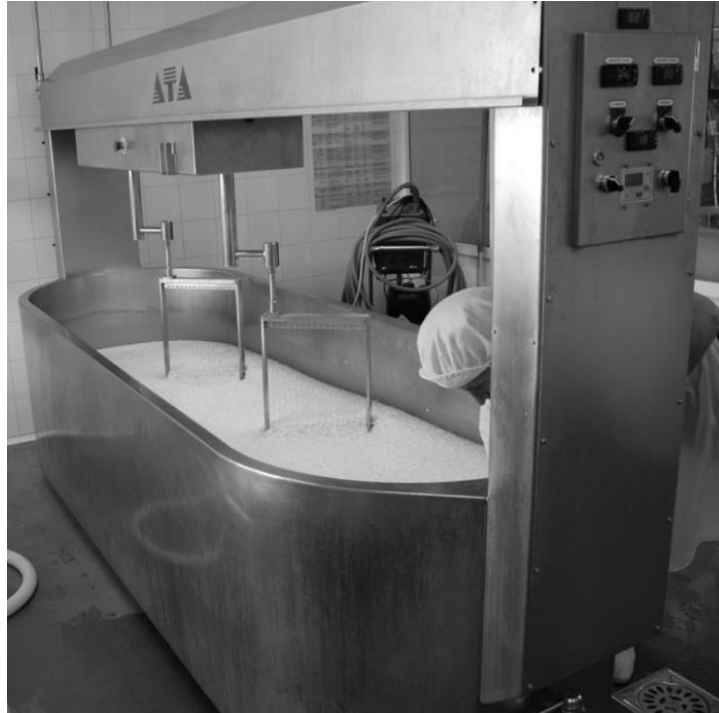
Figure IV.2. Oval-shaped vat with two axes of rotation and cutting frames with vertical wires (Original photo: A. Aldalur).
