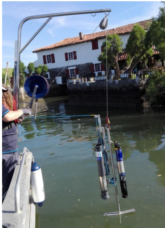
Figure 3.6: Photo of the structure used to collect bottom samples.
