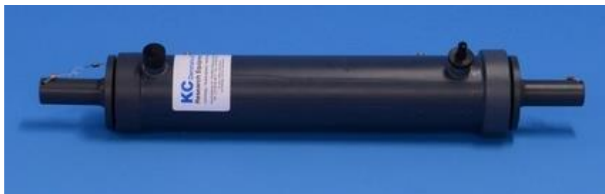
Figure 3.4: Photo of the Niskin sampling bottle used to take bottom samples.
