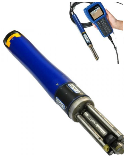
Figure 3.5: Photo of the EXO2 multiparametric probe.
