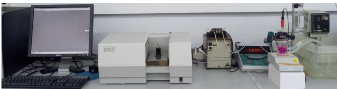
Figure 7.2: Experimental assembly used to simultaneously measure the spectrum and the pH (potentiometrically) of the samples.
