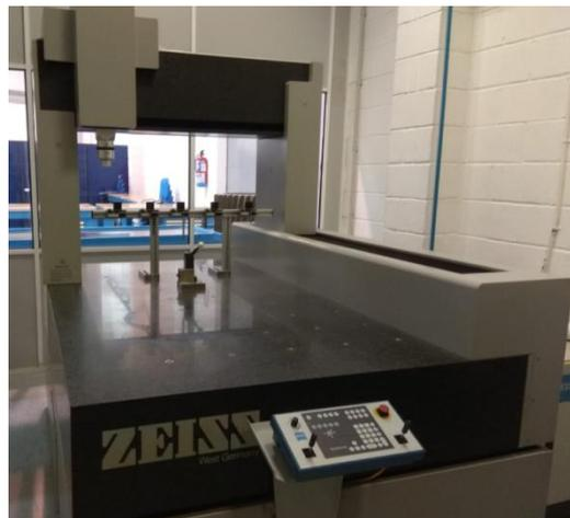
*Figura 31: Máquina C.M.M. ZEISS MC 850.*
