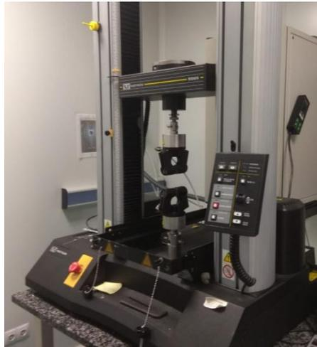
*Figura 29: Máquina Instron 5565.*
