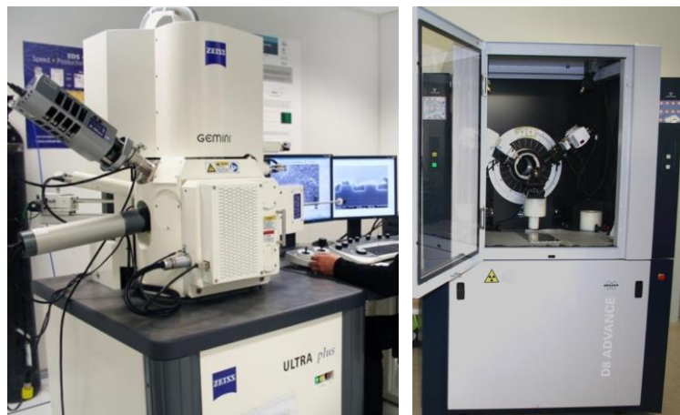
Fig. A.I.6 ZEISS ULTRA plus SEM microscope (left) and D8 Advance X-ray diffractometer (right)
