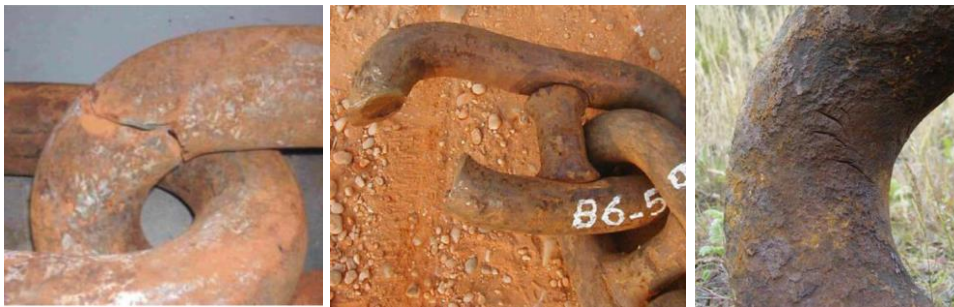
Fig. 2.4 Chain failure by corrosion-fatigue crack propagation in the crown (left [36] and middle [37]), and fatigue crack initiation in the crown (right) [37]
