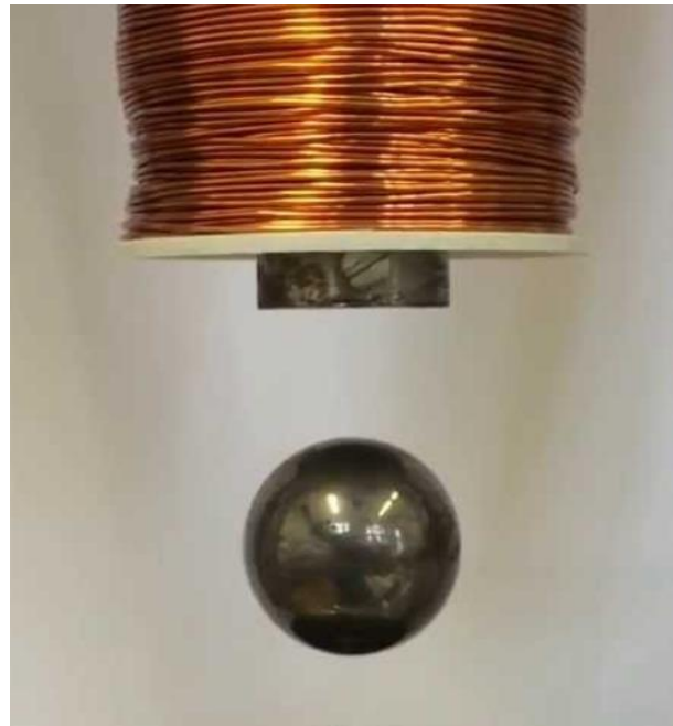
Figure 2 Example of Magnetic Levitation Using an Electromagnet (From [5])
