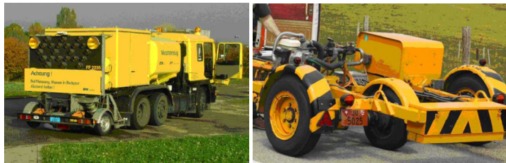
Fig. 3.24. a) SRM mounted on the rear part of the vehicle, b) Skiddometer BV-8 (Do and Roe, 2008).
