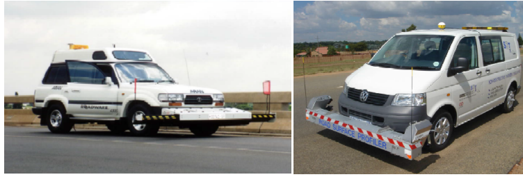
Fig. 3.68. High Speed Inertial Profilers (COTO, 2007).
