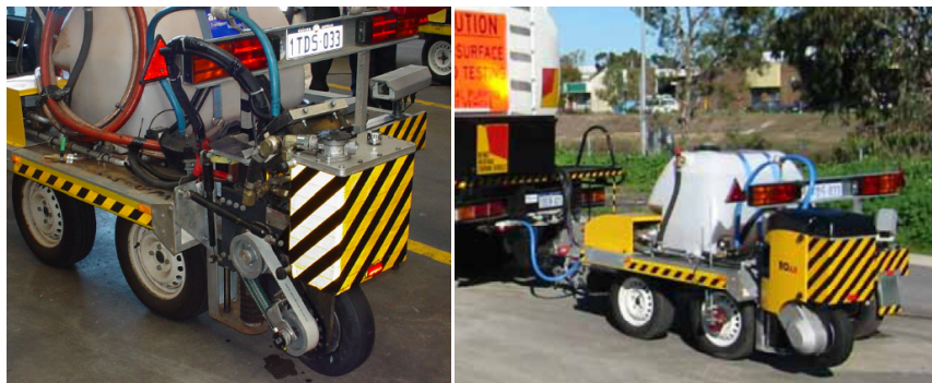
Fig. 3.29. a) ROAR device with testing wheel and hydraulic braking mechanism (Wilson 2006), b) ROAR operating (Austroad, 2011a).
