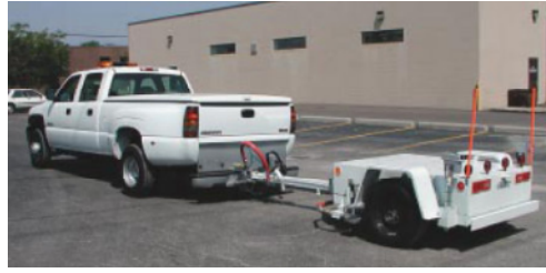
Fig. 3.22. ASTM E-274 locked wheel device, towed by testing vehicle (Wilson, 2006).
