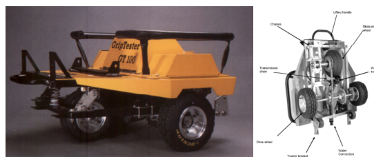
Fig. 3.26. Side view of the Griptestter (left) (Wilson 2006) and Griptestter measuring wheel and chain transmission (right) (Do and Roe, 2008)
