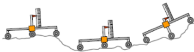
Fig. 3.60. Measuring principle of the rolling straightedge.
