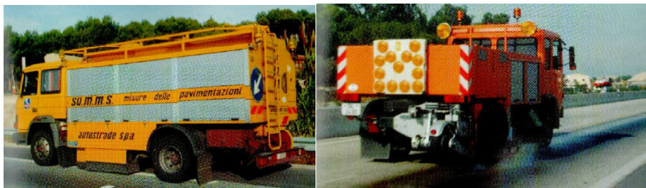
Fig. 3.35. Italian SUMMS, b) German SCRIM/SRM, both at the International Experiment (Achutegi Viada 2005).
