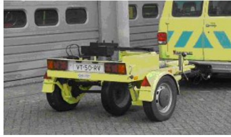
Fig. 3.28. RWS NL skid resistance trailer (Do and Roe, 2008)
