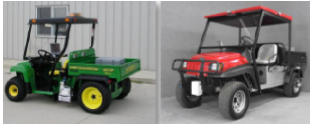
Fig. 3.69. Fig. Lightweight Inertial Profilers (COTO, 2007).
