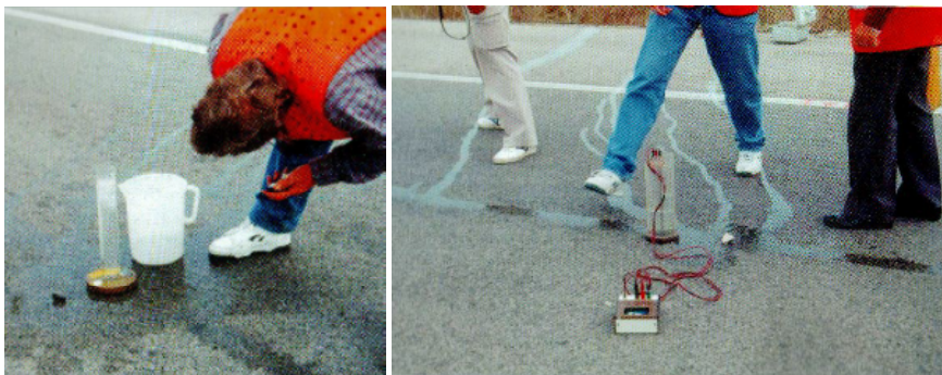
Fig. 3.40. Outflow volumetric test. a) with manual chronometer, b) with automated chronometer Achutegi Viada 2005).
