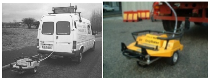
Fig. 3.25. Griptestter operating. (Feighan 2006; Kogbara et al. , 2016).
