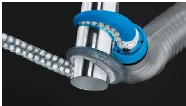
Figura 10: Bionic Handling Assistant (octopus). [13]
